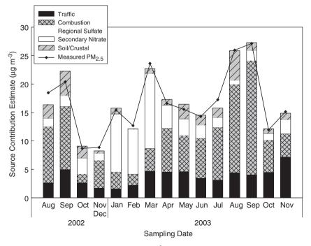
Fig. 8. Monthly average PM<sub>2.5</sub> mass contributions (μg m<sup>-3</sup>) at LPH from the UNMIX-generated source profiles.
