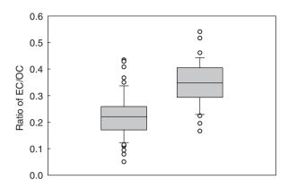
Fig. 2. Box plots of EC/OC ratio at Lower Price Hill (N=68) and Findlay (N=39). Whiskers represent 5th and 95th percentiles with individual data points outside these thresholds denoted by open circles.
