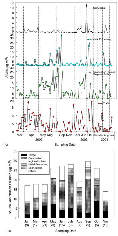
Fig. 7. (A) Daily average of  $PM_{2.5}$  mass contributions ( $\mu g \, m^{-3}$ ) at Findlay from the UNMIX-generated source profiles. (B) Monthly average  $PM_{2.5}$  mass contributions ( $\mu g \, m^{-3}$ ) at Findlay from the UNMIX-generated source profiles.
