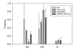
Fig. 6. Comparison of UNMIX-estimated traffic source profiles for various diesel engine emissions measurements. Normalized chemical profiles (sum of the identified weight = 1) of EC, OC, and sulfur.
