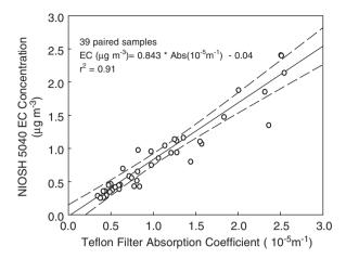
Fig. 4. Plot of measured EC concentration (NIOSH 5040 ECOC analysis on quartz filters) against absorption coefficients from reflectance measurements on Telfon filters for collocated samples. Solid line is the best-fit simple linear regression; dashed lines are the 95% confidence levels.
