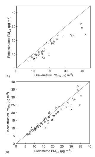
Fig. 3. Plot of reconstructed  $PM_{2.5}$  mass concentrations based on speciated measurements against the gravimetric  $PM_{2.5}$  mass concentrations: (A) Findlay; and (B) LPH. The solid line is the 1:1 line. Samples deemed outliers for the purpose of UNMIX modeling are denoted by ' $\times$ '.
